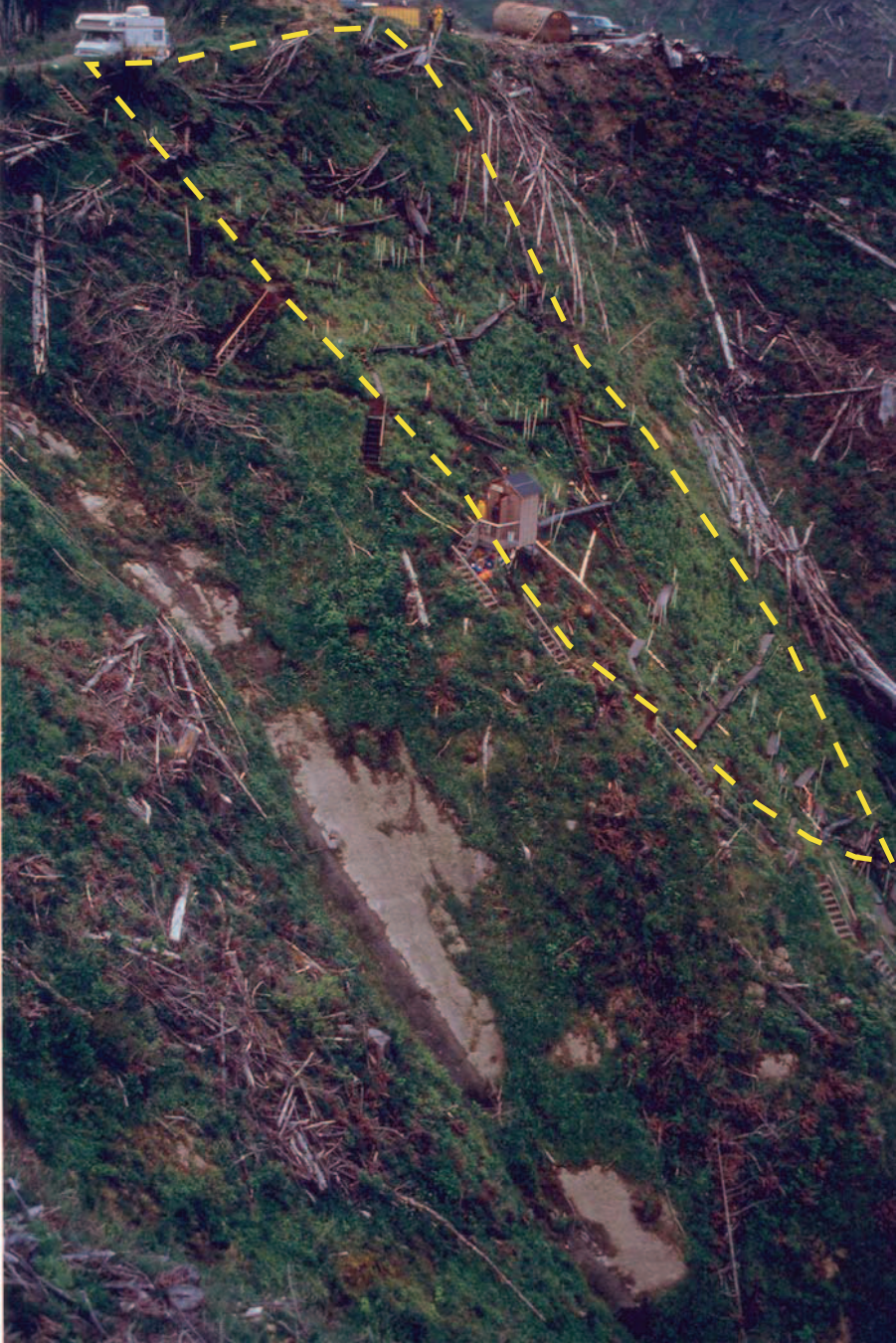
Fig. 2. Photograph of CB1 showing stairs / platforms, water tank, piezometers, shed that housed the TDR multiplexer, and a landslide scar in the adjacent hollow (bottom left).
