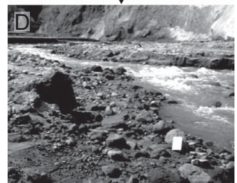
Figure 15. Development of bed armor in Pinatubo channels from (A) unarmored through (B) development of pebble clusters to (C) partial armor layer covering active channel surface as pebble clusters begin to interact to (D) fairly complete armor layer following incision during the dry season. Gravelometer for scale in (A) and (B) is 340 \times 280 mm. Field book for scale in (C) and (D) is 120 \times 195 mm.
